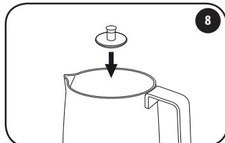
Place the smooth disk for mixing over the pin inside the jug. The smooth disk is housed beneath the motor base.
