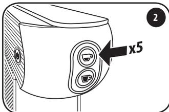
With the machine off, press the ☕ button 5 times to access the temperature change function. The ☕ and ☕ buttons will begin to flash.
