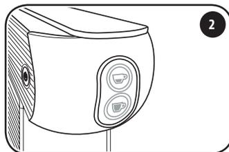
2 When buttons ☕ and ☕ are illuminated and unblinking, the machine is ready to be used.
