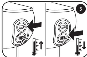
Press the ☕ button to increase the temperature by 3 degrees. Press the ☕ button to decrease the temperature by 3 degrees.
