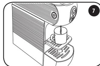
**CAUTION:** Wait at least 5 seconds after dispensing before lifting the lever. After delivering 10 successive cups of coffee, wait for at least 2 minutes before preparing another coffee. The machine is designed for single deliveries with a maximum duration of 75 seconds.
