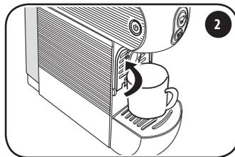
2 To use large cups, close the support and place the cup directly on the drip tray.
