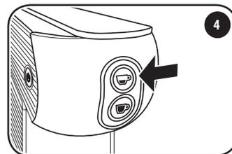
4 Press the ☕ button; the machine will dispense water; press the ☕ button again. The rinsing operation is completed when at least three cups of water have been delivered.
