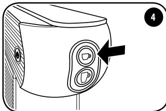
Press the ☪button; the machine will dispense water; press the ☪button again. The rinsing operation is completed when at least three cups of water have been delivered.
