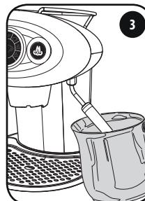
Press the steam button ; the steam symbol on the dial lights up to indicate that the machine is preparing to enter "steam" mode.
