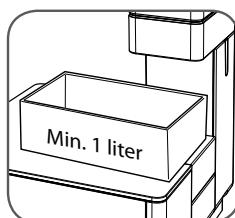
Place a container with a capacity of at least 1 litre beneath the brew group "C".
