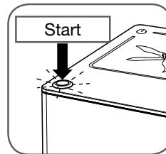
Run water through the machine by pressing the coffee button.
