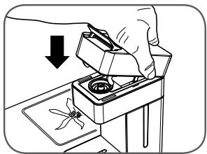
Lower the movable part of the top of the machine completely, and press the lever "A" until you hear it lock in place.
