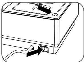
Move the main on/off switch "M" into the "I" position. The indicator LED "D" will light up.
