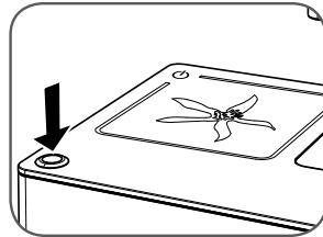
The machine will start warming up; the temperature ready LED of the coffee button "F" will remain off.
