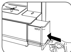
After setting the lid back in place, insert the tank completely into the machine until it clicks firmly into place.
