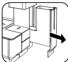
Remove the used capsule container "G" by pulling it out.
