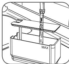
Remove the water tank "L" and lid and wash them under running water.
