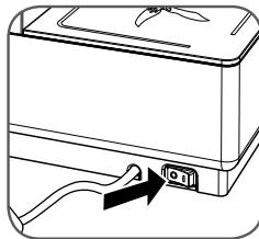
Switch the machine off and disconnect the plug from the power outlet.
