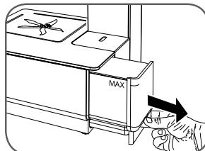
Remove the water tank "L" from the machine by pulling it slightly up and then out.
