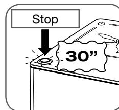
After 30 seconds press the coffee button "F" again to shut off the flow.
