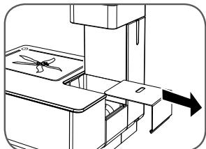
To adjust the height of the cup stand "H" you must remove it by pulling it out and then set it in the mug or espresso cup position.
