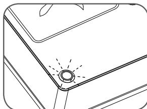
Make sure the temperature OK indicator "F" is on. Do not make coffee if the indicator "F" is off.
