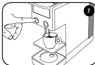
Press and release the ☕ button. The appliance will stop dispensing automatically.
