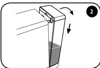
Remove the tank and empty the remaining water.
