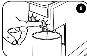
Place a container of at least 0.75 litre capacity under the dispensing spout.
