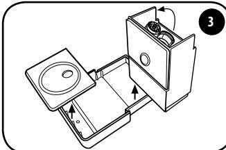
Empty the capsule holder and rinse it. Clean the drip tray and the grid to remove residue of water and coffee. Once clean, engage the tray in the grid.
