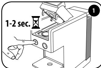
With the lever open, turn on the machine by pressing one of the two coffee buttons for 1-2 sec.
