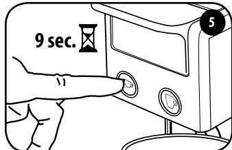
Turn on the machine by pressing the button for 9 seconds.
