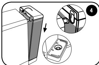
Reinsert the tank where the two slots are and push it towards the machine until fully engaged.
