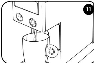
Press the ☕ or ☪ button and wait until the water stops dispensing. The machine is rinsed when at least 3 mugs of water have been dispensed. The machine is now ready for use.
