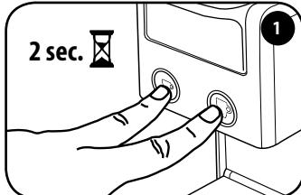
Switch off the machine by pressing the two coffee ☕️ keys simultaneously for 2 seconds.
