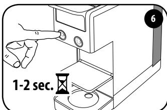
Turn on the machine by pressing one of the two coffee buttons for 1-2 sec.
